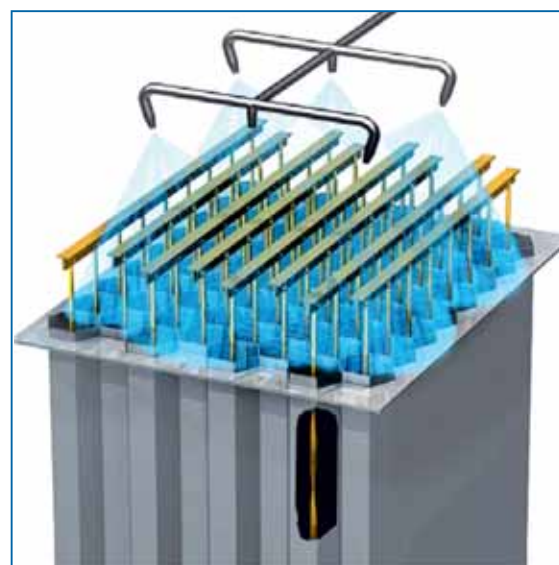
Electrodes cleaned by periodic flushing system
